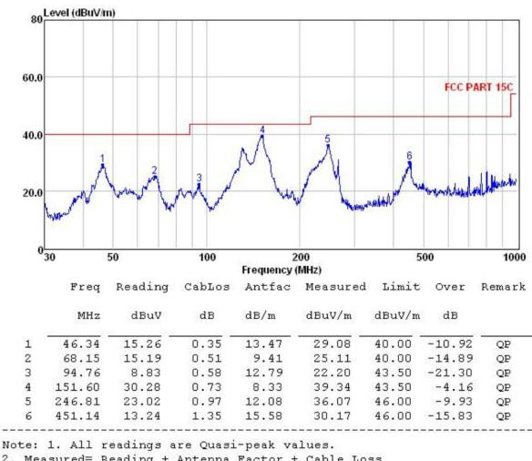
2. Measured= Reading + Antenna Factor + Cable Loss
