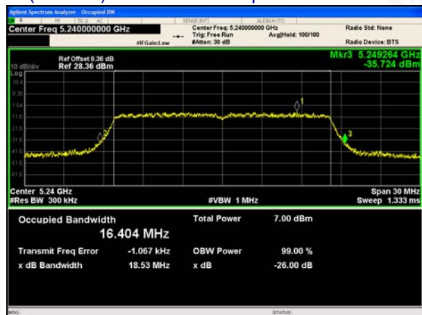
(802.11a) 26dB Bandwidth plot on channel 48
