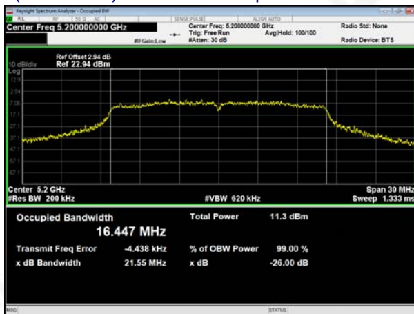
(802.11 n20) 99% Bandwidth plot on channel 40
