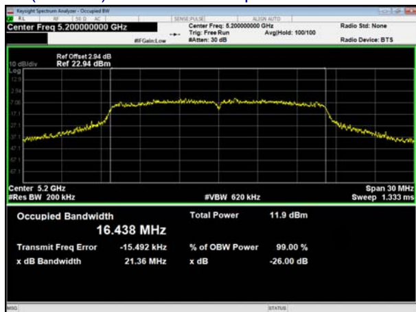
(802.11a) 99% Bandwidth plot on channel 40
