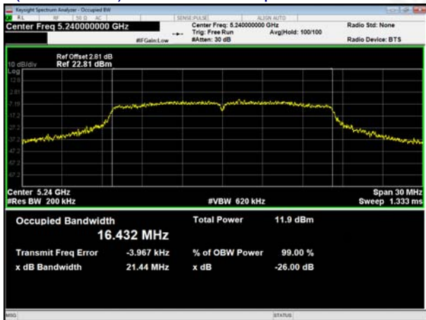
(802.11ac20) 99% Bandwidth plot on channel 48
