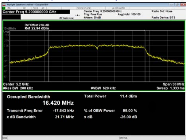
(802.11ac20) 99% Bandwidth plot on channel 40
