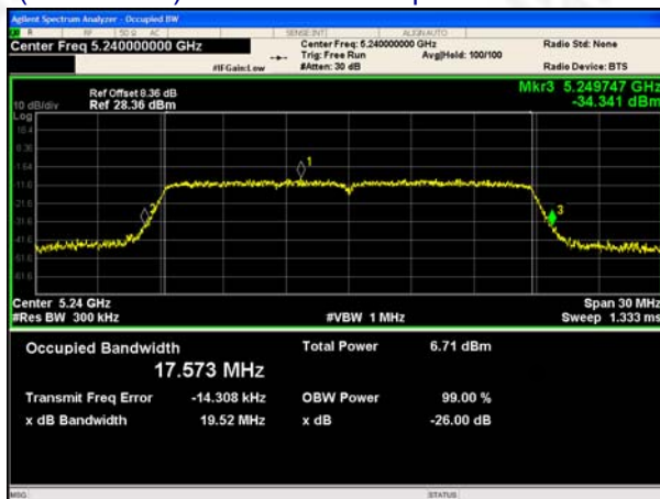
(802.11 n20) 26dB Bandwidth plot on channel 48
