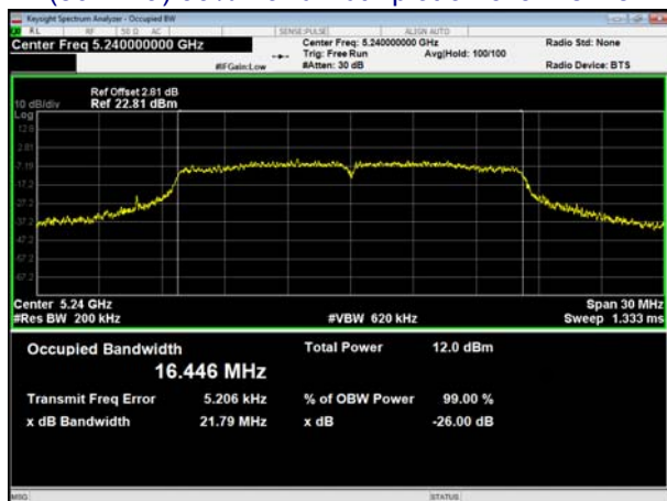
(802.11a) 99% Bandwidth plot on channel 48
