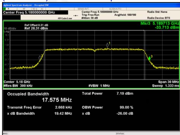
(802.11ac20) 26dB Bandwidth plot on channel 36
