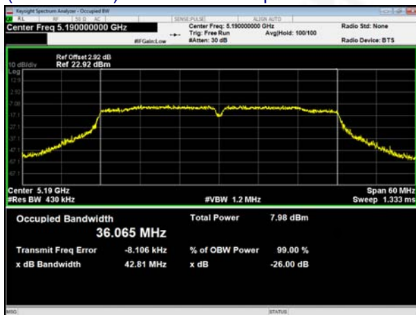
(802.11 ac40) 26dB Bandwidth plot on channel 38
