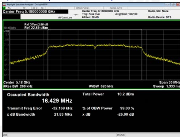
(802.11 n20) 99% Bandwidth plot on channel 36
