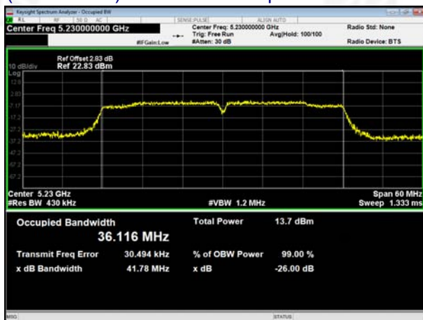
(802.11 ac40) 26dB Bandwidth plot on channel 46
