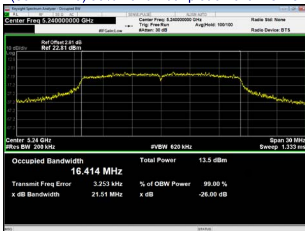
(802.11 n20) 99% Bandwidth plot on channel 48
