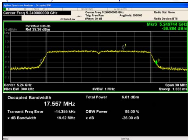
(802.11ac20) 26dB Bandwidth plot on channel 48
