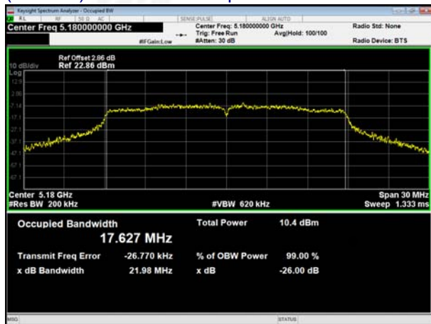
(802.11a) 99% Bandwidth plot on channel 36
