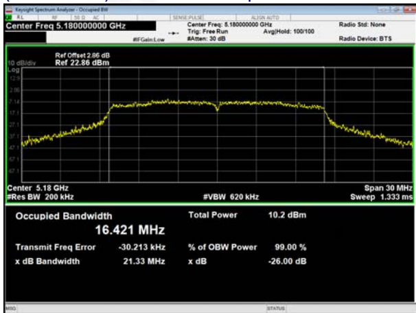
(802.11ac20) 99% Bandwidth plot on channel 36
