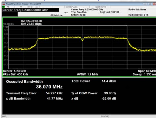
(802.11 ac40) 99% Bandwidth plot on channel 46
