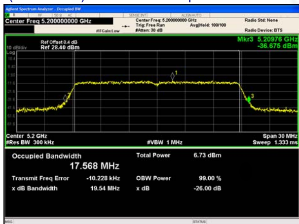
(802.11ac20) 26dB Bandwidth plot on channel 40
