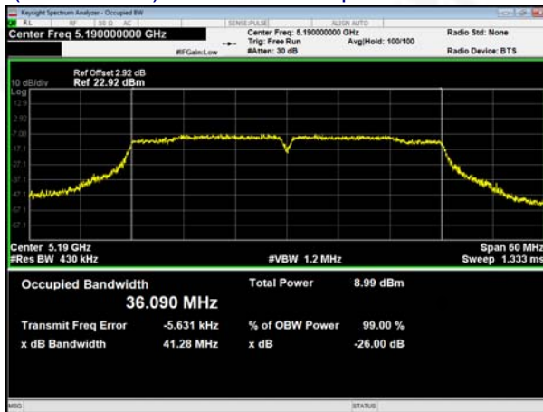
(802.11 ac40) 99% Bandwidth plot on channel 38
