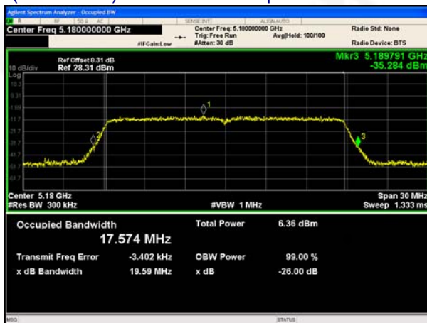
(802.11 n20) 26dB Bandwidth plot on channel 36
