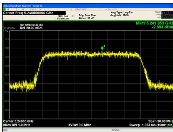
(802.11n20) PSD plot on channel 48
