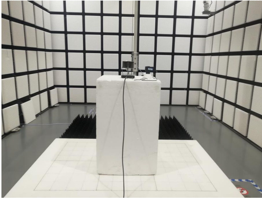
Fig. 3 Radiated emission setup photo(Above 1GHz)
