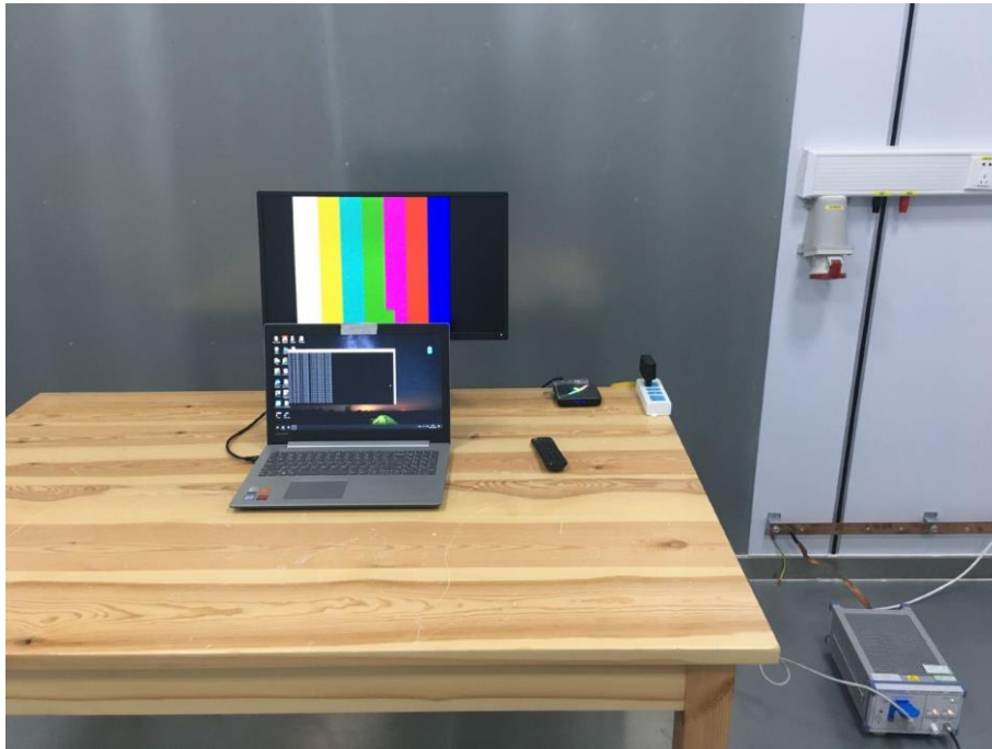
Fig. 4 Power line conducted emission setup photo
