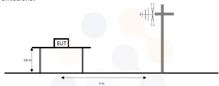
The diagram below shows the test setup that is utilized to make the measurements for emission from 1  $\oplus$  to 40  $\oplus$  emissions.
