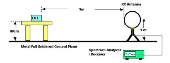
For Radiated Emissions: 30MHz~1GHz
