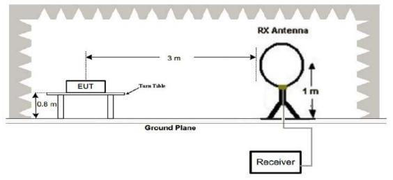
(2) Radiated Emission Test-Up Frequency 30MHz~1GHz
