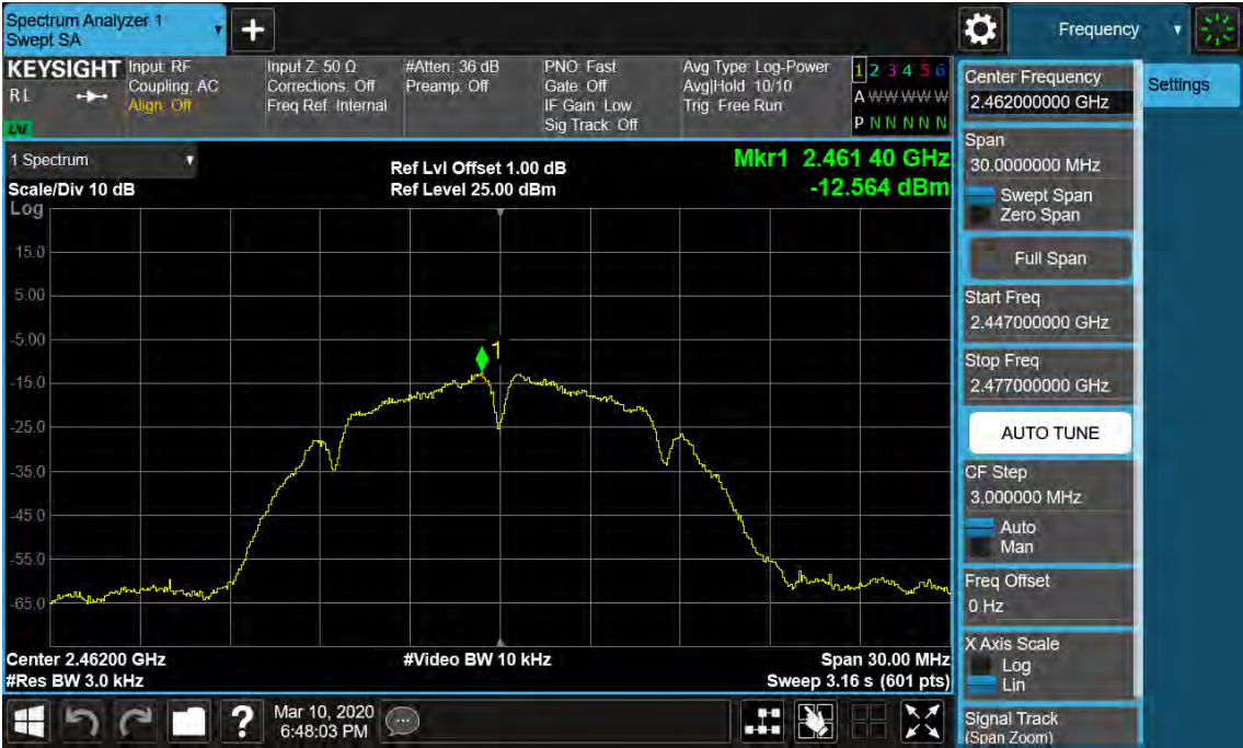
Figure 12: Power Spectral Density, 802.11b, 2462MHz
