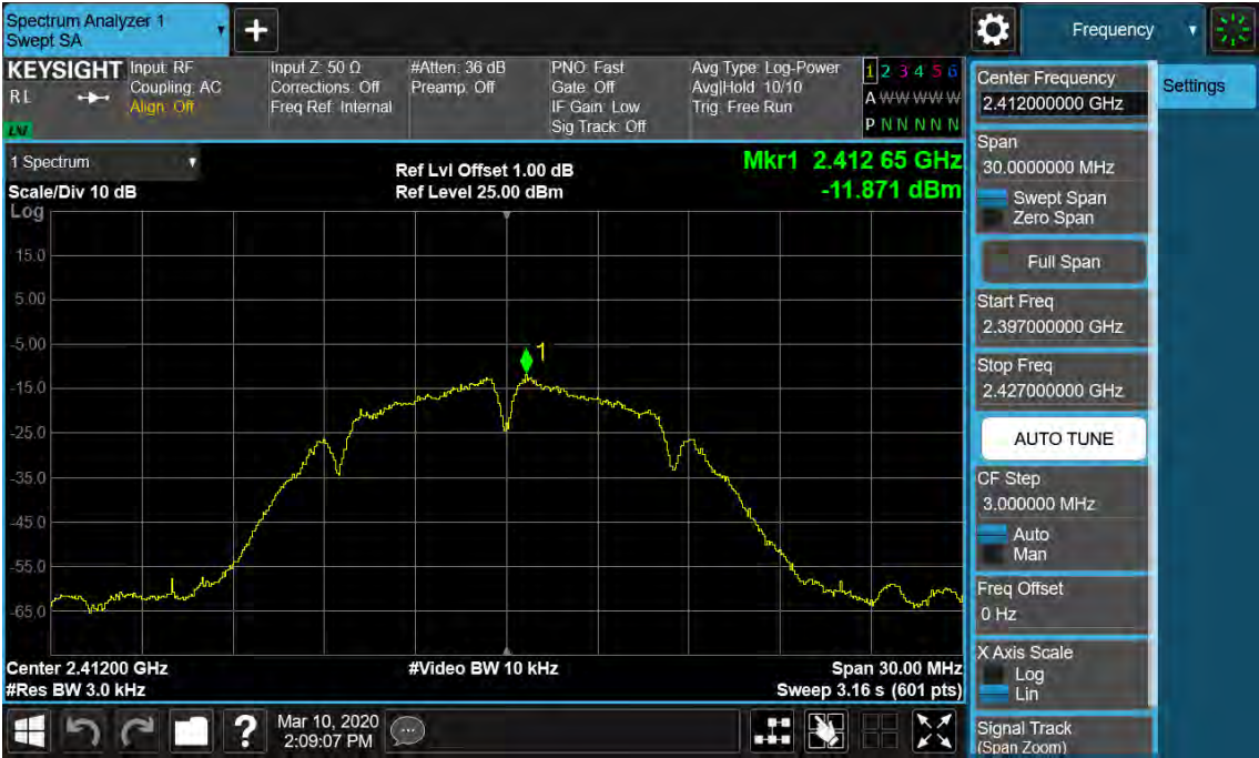
Figure 10: Power Spectral Density, 802.11b, 2412MHz
