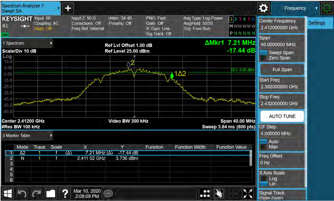
Figure 1: 6dB Bandwidth and 99% Bandwidth, 802.11b, 2412MHz
