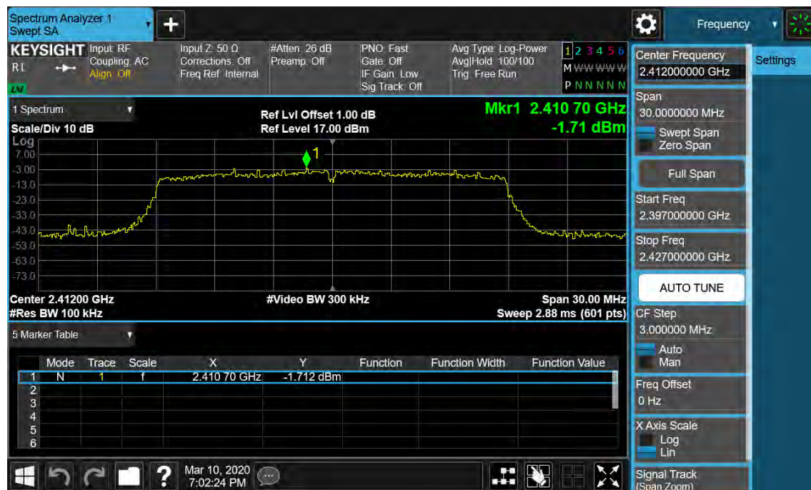
Figure 25: Conducted Spurious Emission & Authorized-band band-edge, 802.11n(HT20), 2412MHz Carrier Level
