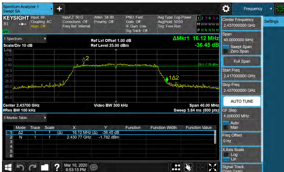
Figure 5: 6dB Bandwidth and 99% Bandwidth, 802.11g, 2437MHz
