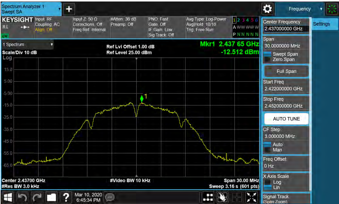
Figure 11: Power Spectral Density, 802.11b, 2437MHz
