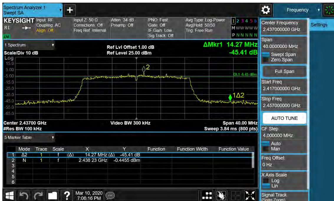
Figure 8: 6dB Bandwidth and 99% Bandwidth, 802.11n(HT20), 2437MHz
