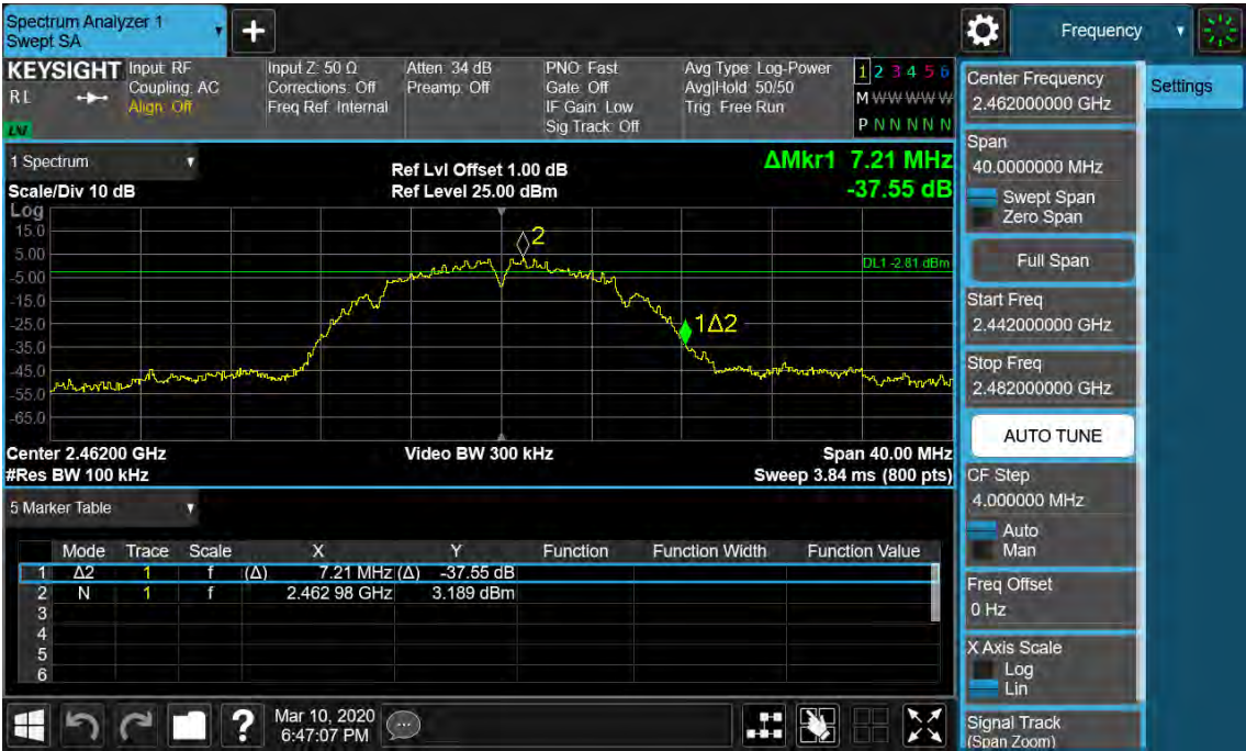
Figure 3: 6dB Bandwidth and 99% Bandwidth, 802.11b, 2462MHz
