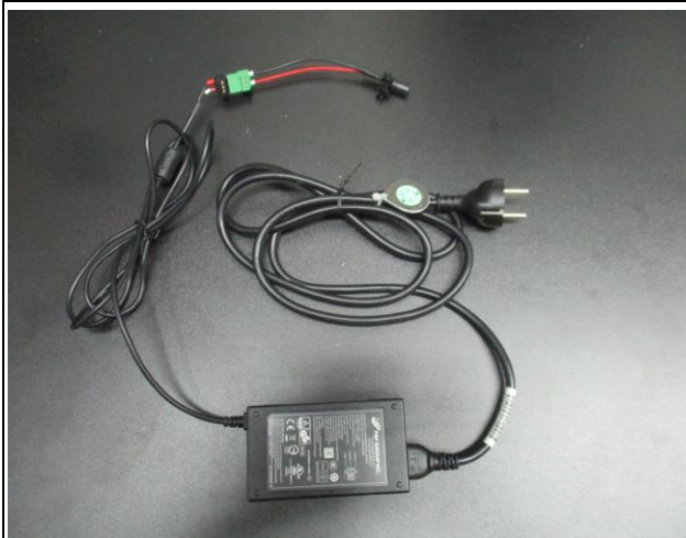
Interface X2 Power cable EUT, PSU FSP is AE and not part of the EUT
