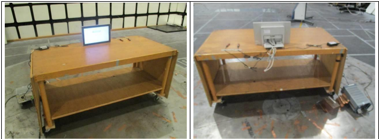
Figure 6-1: test setup Low voltage AC mains continuous disturbance
