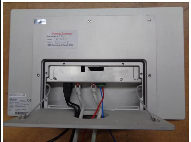
Rear view of Touch-it CE VESA glass 15,6 (open case)
