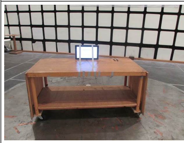
Figure 2: test setup Radiated disturbances 30 MHz to 1000 MHz
