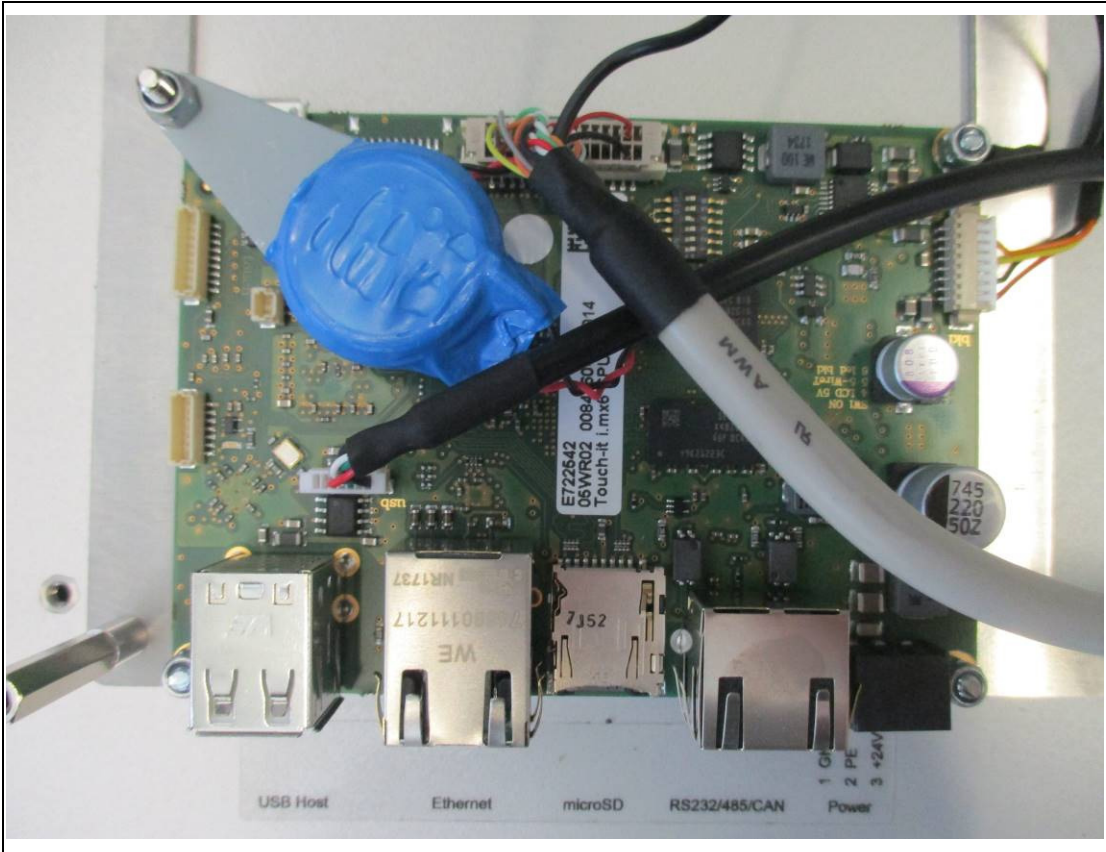
Figure 2: Front view of Main board of Touch-it CE Front Panel glass 15,6
