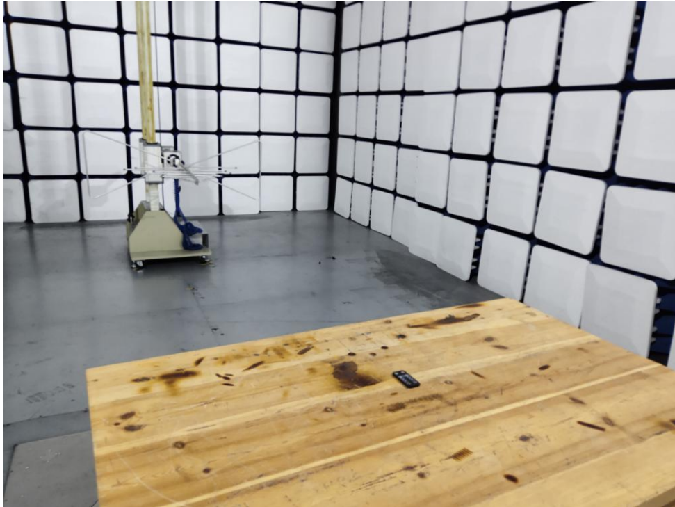
Photo of Radiated Emission Measurement
