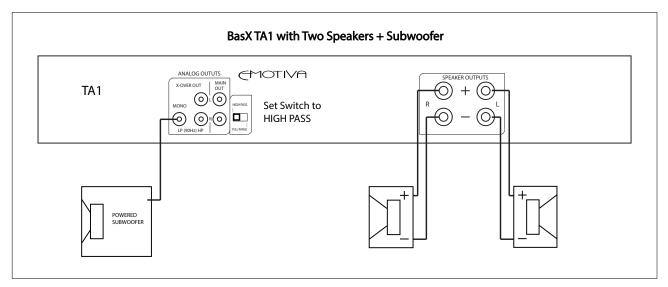
Note: The active bass management high-pass filter is always applied to the HP Xover-Out outputs on the TA1. The setting of the Crossover Switch controls whether the active high-pass filter is applied to BOTH THE MAIN OUTPUTS AND THE SPEAKER OUTPUTS.
