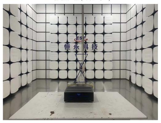
**Radiated Test (Above 1GHz)**
