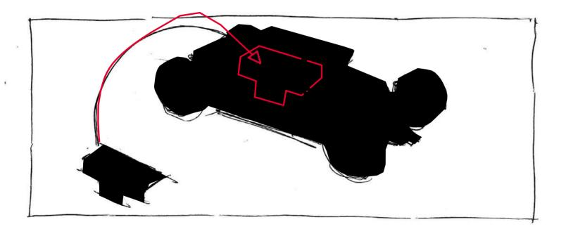
Slide the battery compartment cover over the battery until it clicks.
