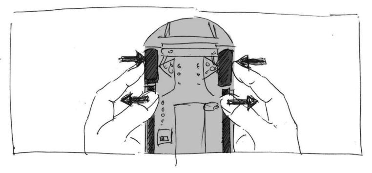
Detach the body from the chassis by spreading the rear side sills from below with your thumb. Hold the rear wheels with your index fingers while lifting the motor bracket forward.
