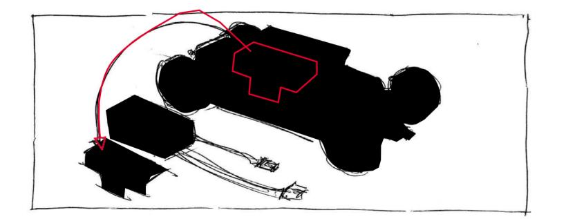
Remove the cover of the battery compartment with an audible click.
