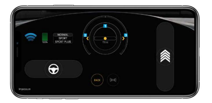
To ensure precise straight-line stability, it may be necessary to readjust the trim 1.
