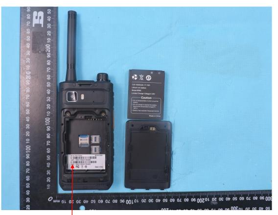
20mm Multi Mode 4G Android PTT Phone Model name: E966 FCC ID: 2AVAF-E966 This device complies with part 15 of the FCC Rules. Operation is subject to the following two conditions: (1) This device may not cause harmful interference, and (2) this device must accept any interference received, including interference that may cause undesired operation.
