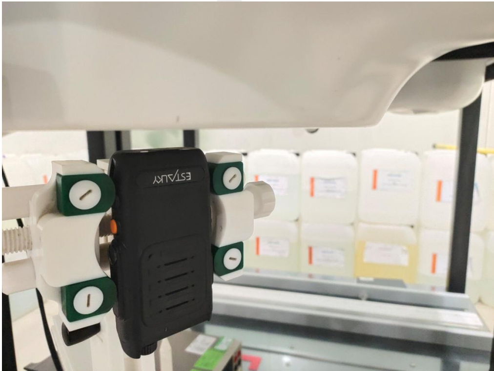
Bottom Edge(separation distance is 10mm)
