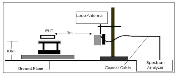
(B) Radiated Emission Test-Up Frequency 30MHz~1GHz
