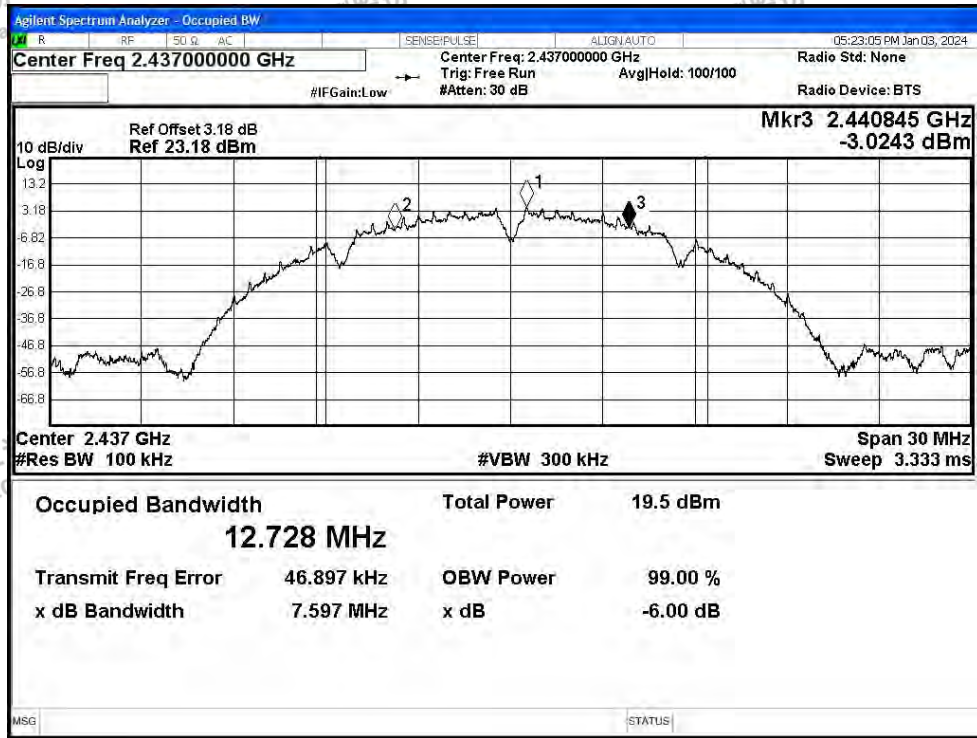
-6dB Bandwidth NVNT b 2437MHz Ant1
