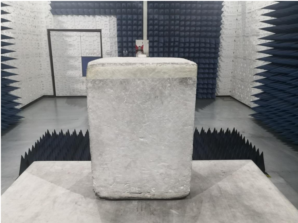
RADIATED EMISSION TEST SETUP ABOVE 1GHZ
