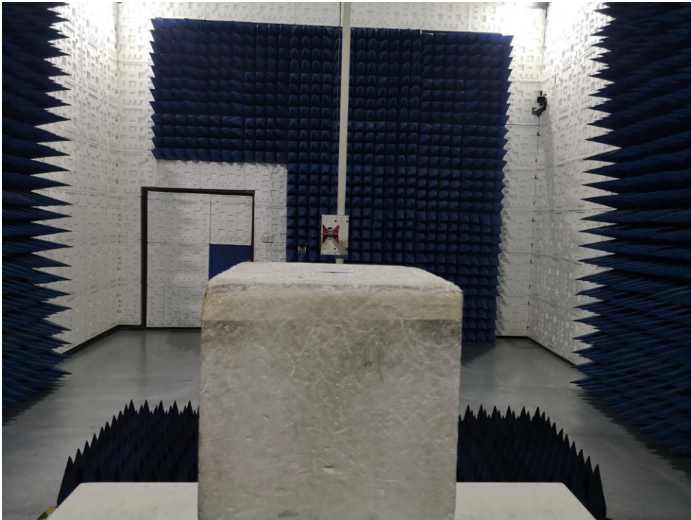
RADIATED EMISSION TEST SETUP ABOVE 1GHZ
