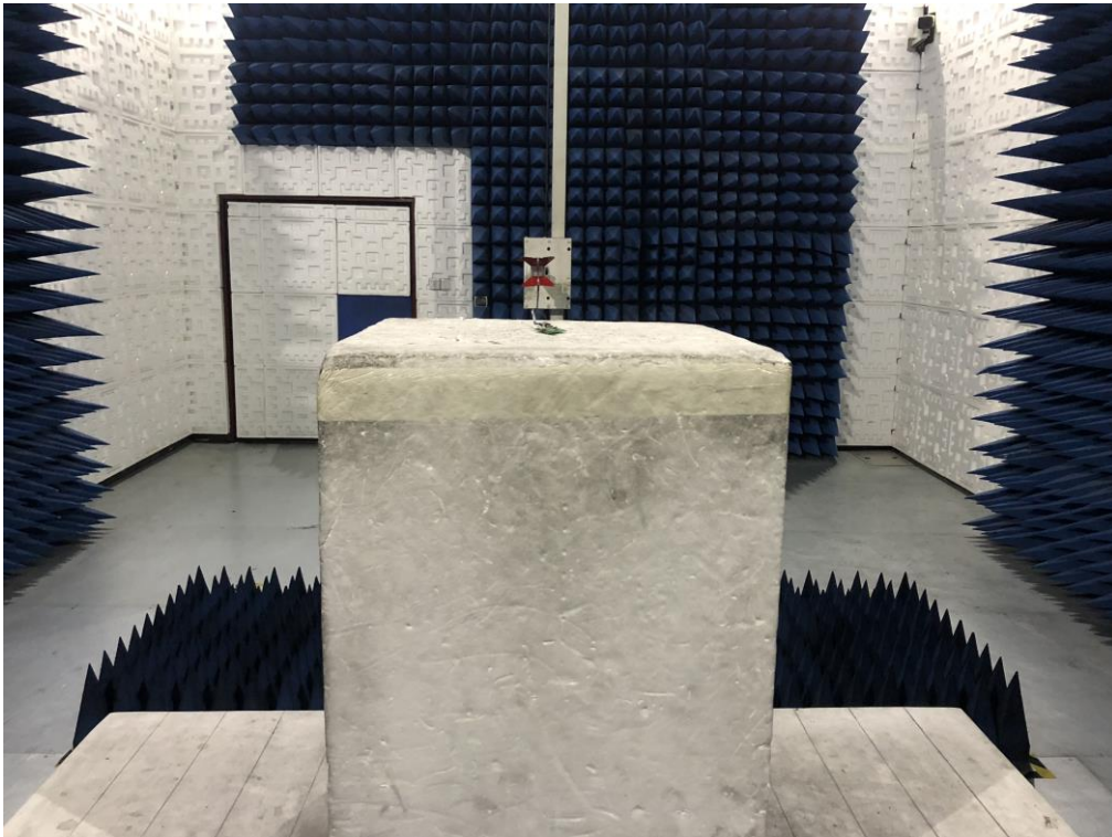
RADIATED EMISSION TEST SETUP ABOVE 1GHZ
