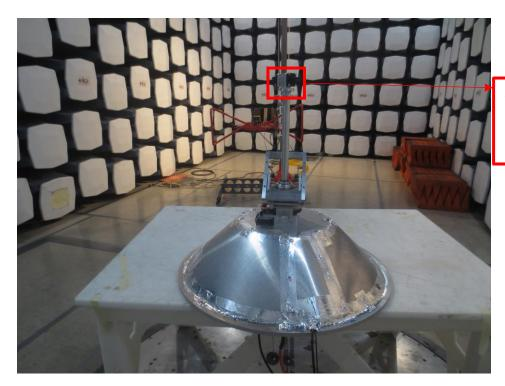
Antenna port was terminated with waveguide adapter and 50 ohm load.
