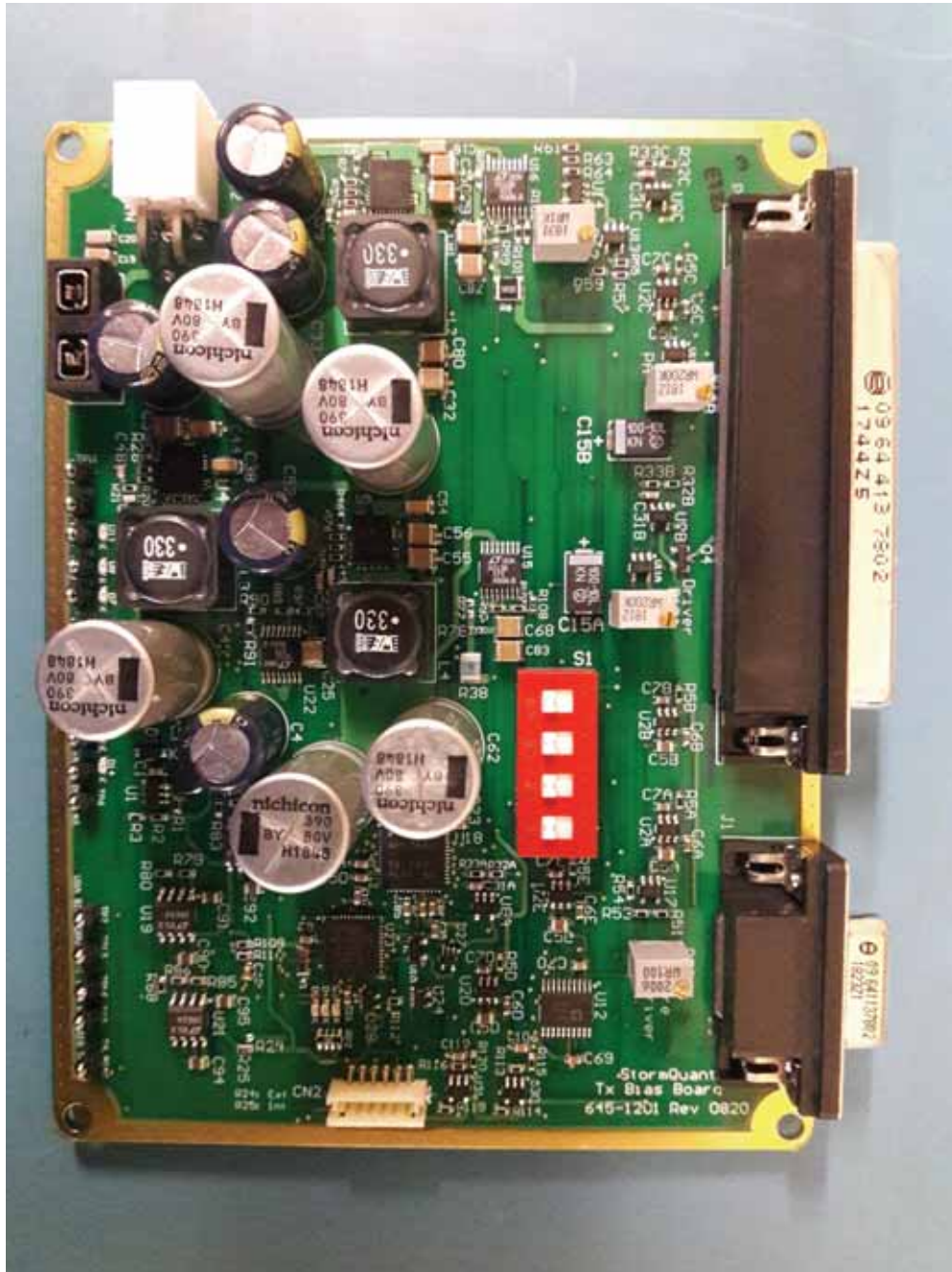
Transmitter BIAS Board, Frontside
