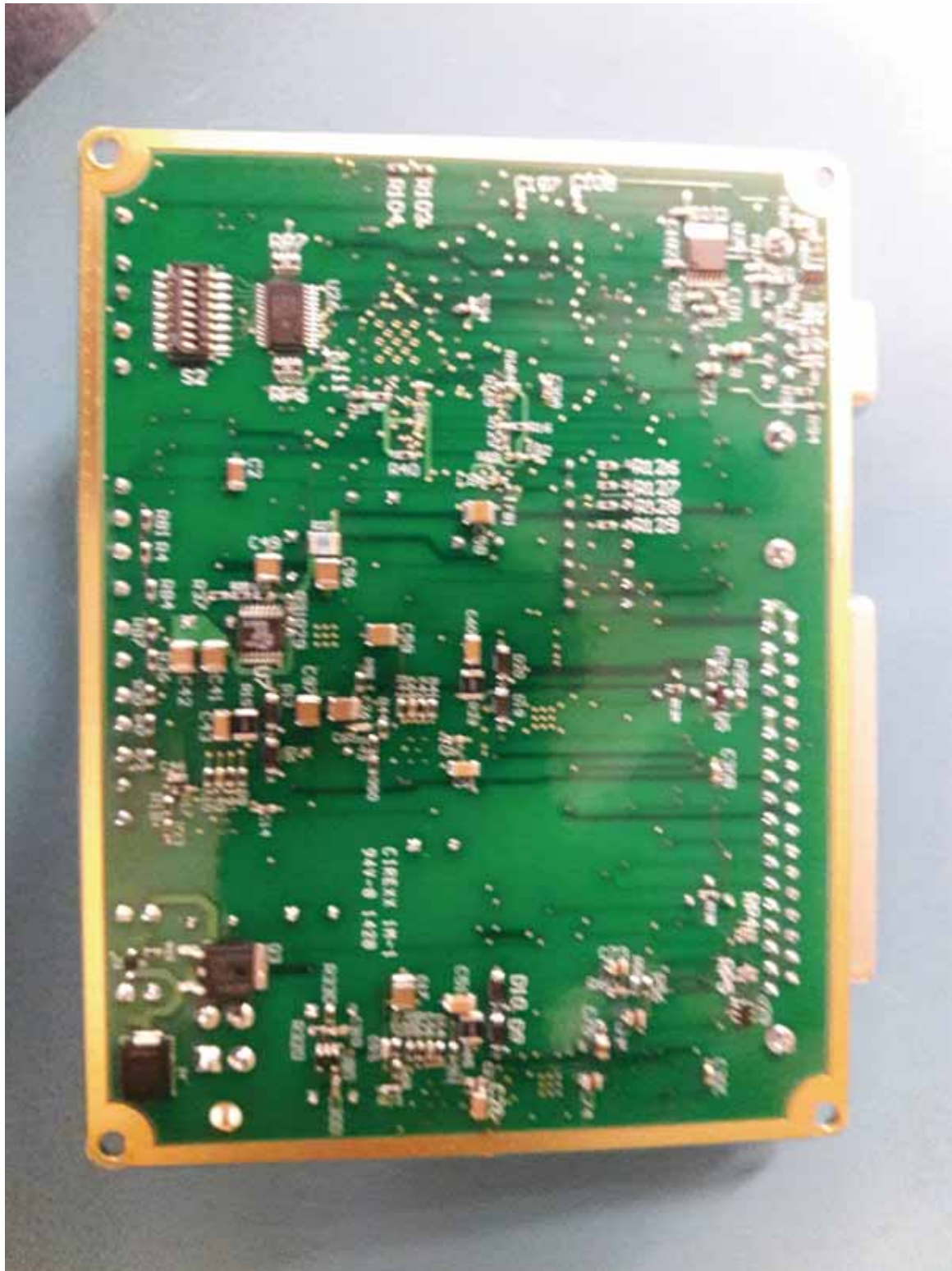
Transmitter BIAS Board, Backside
