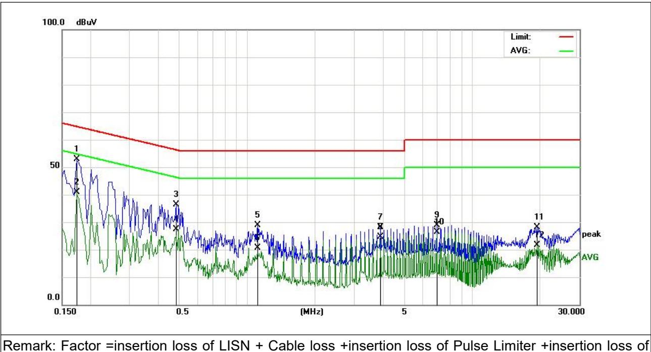
Remark: Factor =insertion loss of LISN + Cable loss +insertion loss of Pulse Limiter +insertion loss of Switch.
