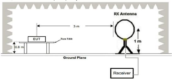
2. Radiated Emission Test-Up Frequency 30MHz~1GHz
