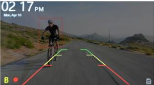
Via the BSD technology, using the image of rear camera to identify the pedestrian position and set the alarm system.
