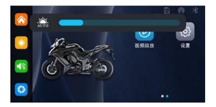
The built-in light sensor at the bottom left of the machine can automatically recognize the brightness of the surrounding environment and adjust the screen brightness to improve comfort. In automatic brightness mode, the brightness can't be manually adjusted.
