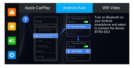
As shown in the picture, click the Android auto button, then select the Android auto option. First, open the WIFI and bluetooth on your phone, as shown in the picture. The bluetooth will automatically turn on and the name will be BRTX-XXX. Once the bluetooth is successfully connected, you can connect to the Android auto system. (when the machine is turned on, it will try to automatically connect to the last connected phone)
