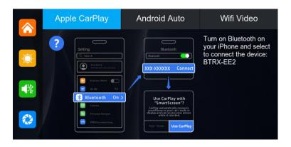
As shown in the picture, click the Apple Caplay button, then select the Apply carplay option. First, open the WiFi and bluetooth on your phone, as shown in the picture. The machine's bluetooth will automatically turn on and the name will be BTRX-XXX. Once the bluetooth connection is successful, apple carplay can be connected. (when the machine is powered on, it will try to automatically connect to the last connected phone)
