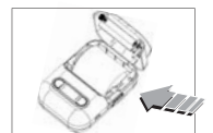
Place the paper roll as shown and Put the print side face down.
