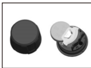
D、取出旧电池并装上新电池(正 极朝上),最后按照安装步骤 重新将传感器安装好 Remove the old battery and install a new one (positive pole upward), then reinstall the sensor according to the Inta- llation steps above
