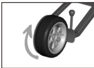
C、松开轮胎 Loosen the tire
