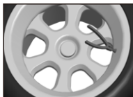
E、用钳子拆下原轮胎气嘴 Remove the original tire nozzle with pliers
