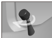
B、拧紧传感器 Screw the sensors tightly
