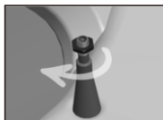
A、拧入防盗六角螺母 Screw the nuts to the bottom of the valve core
