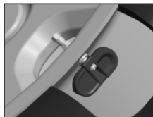
F、将阀杆放入阀门孔中。借助套筒扳手用4Nm拧紧螺母，并用3Nm拧紧螺丝钉。 Place the valve rod into the valve hole; tighten the nut with a socket wrench of 4Nm, and tighten the screw with 3Nm
