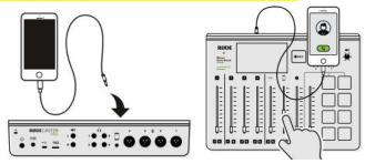
**Step 1:** Connect your smartphone/tablet to Line In/Out jack **(USB port)** on the back using a 3.5mm cable (not supplied) or supplied USB cable.
