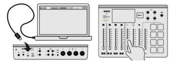
**Step 1:** Connect your PC/MAC to the USB jack on the back using a supplied USB cable. (知道是什么接口的吗)
