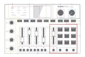
With 27 sample pads (9x3Banks) on the Donner's Podsoler, you can play the preset sound and flexibly record new samples you like during a podcast. It is convenient for players to use and especially adds super fun to the podcast.
