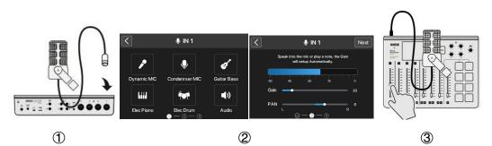
**Step 1:** Connect your microphone to the XLR Input 1-4 jacks on the back using a standard XLR cable (not supplied). Or connect your musical instrument to the XLR Input 1-4 jacks on the back using a standard TRS cable (not supplied).
