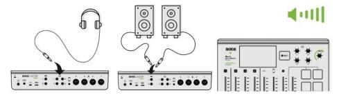
**Step 1:** Make sure to adjust the knob on this unit to a minimum before connecting audio equipment. **Step 2:** Connect your monitor headphones/ monitor speakers to the Main out jacks on the back using a 6.35mm audio cable (not supplied).
