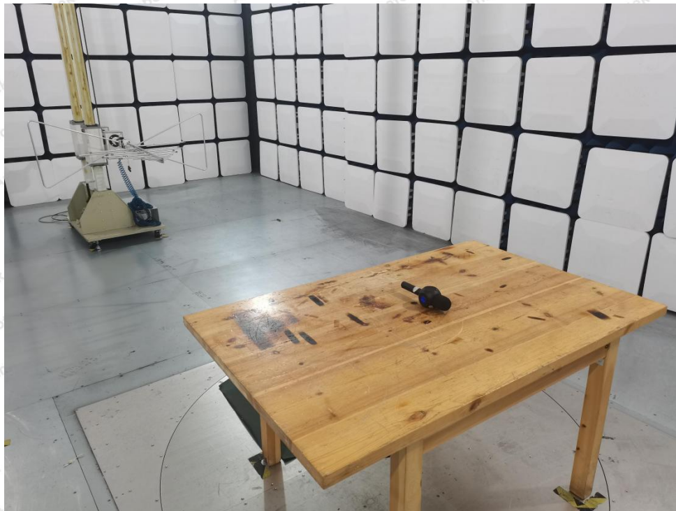
Photo of Radiation Emission Test
