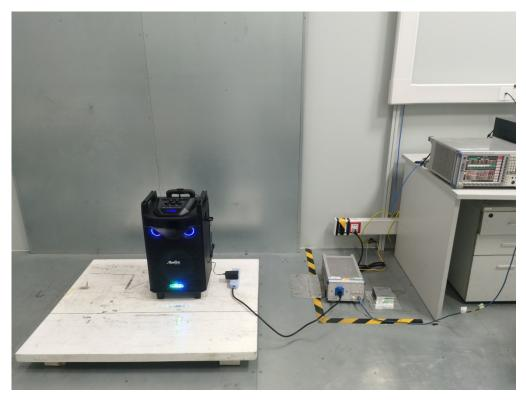
Radiated emission test 30MHz – 1GHz
