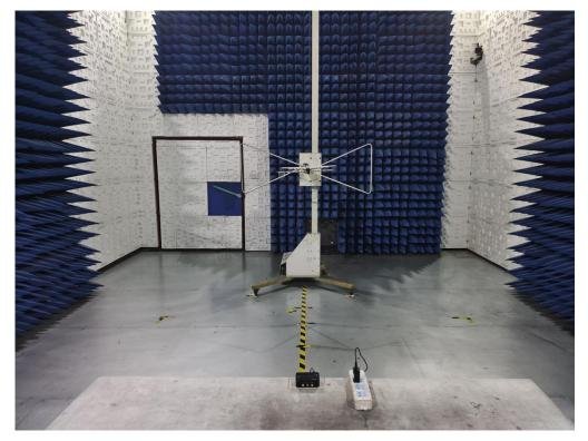
RADIATED EMISSION TEST SETUP ABOVE 1GHz
