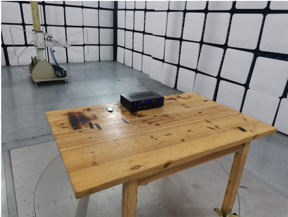
Photo of Radiation Emission Test
