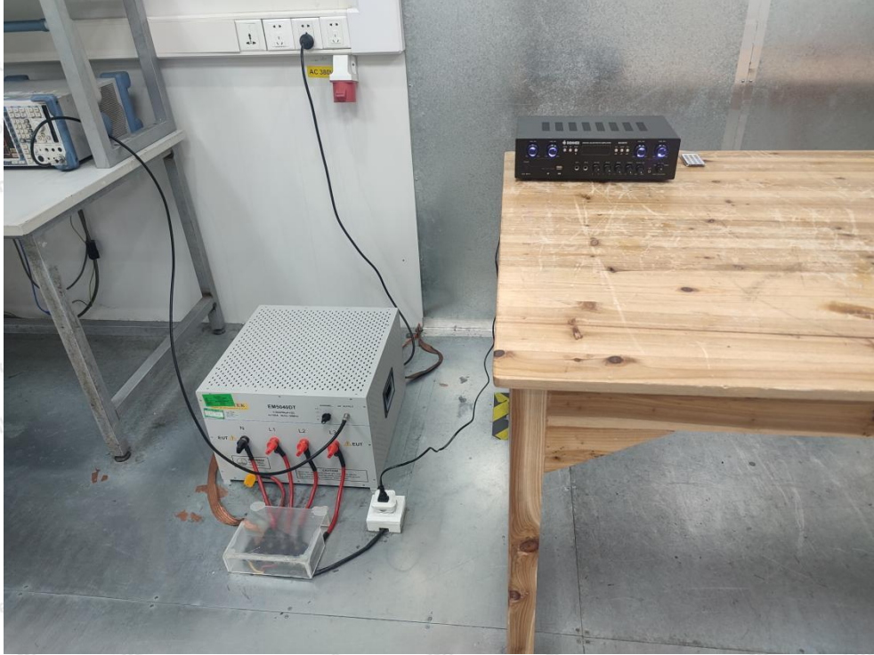
Photo of Conducted Emission Measurement
