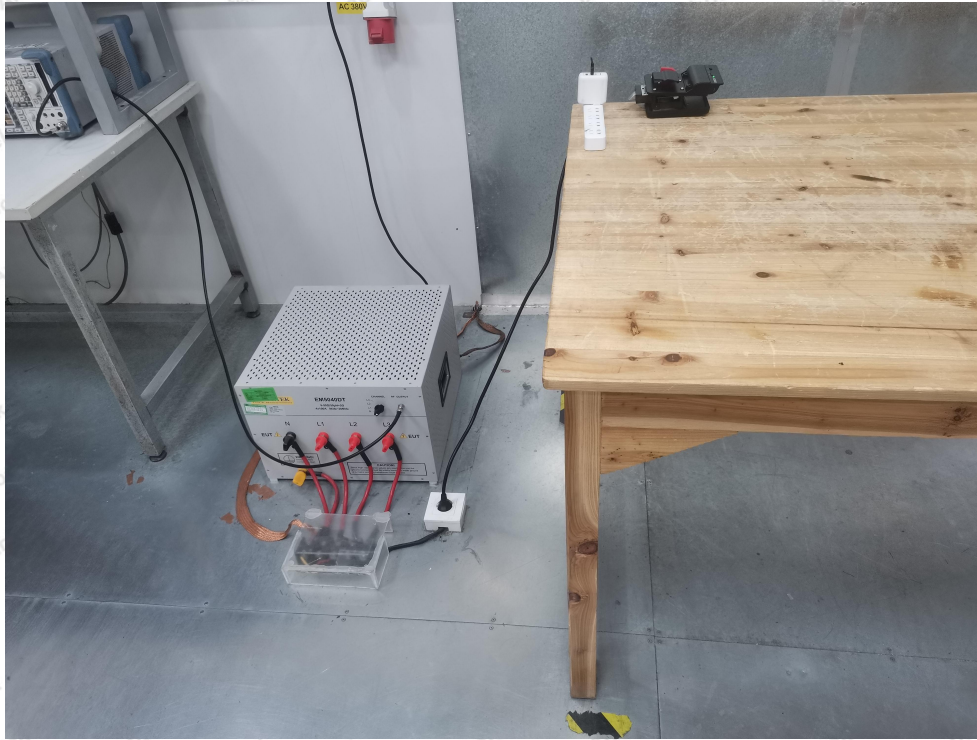
Photo of Conducted Emission Measurement
