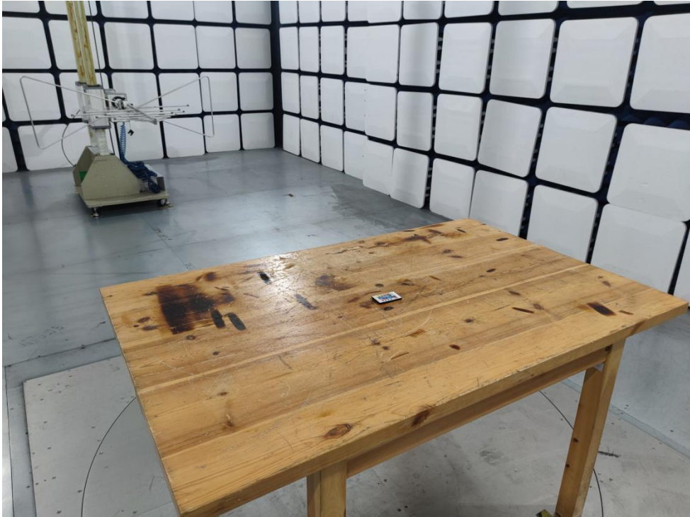
Photo of Radiation Emission Test
