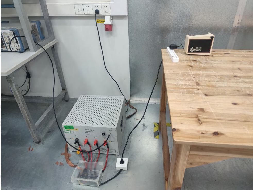
Photo of Conducted Emission Measurement
