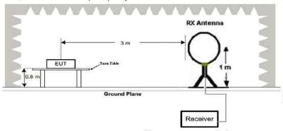
2. Radiated Emission Test-Up Frequency 30MHz~1GHz
