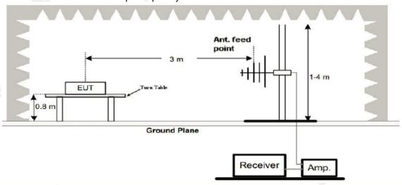
3. Radiated Emission Test-Up Frequency Above 1GHz
