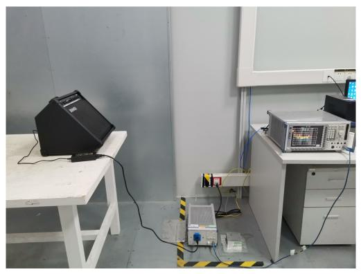
Radiated emission test 30MHz – 1GHz
