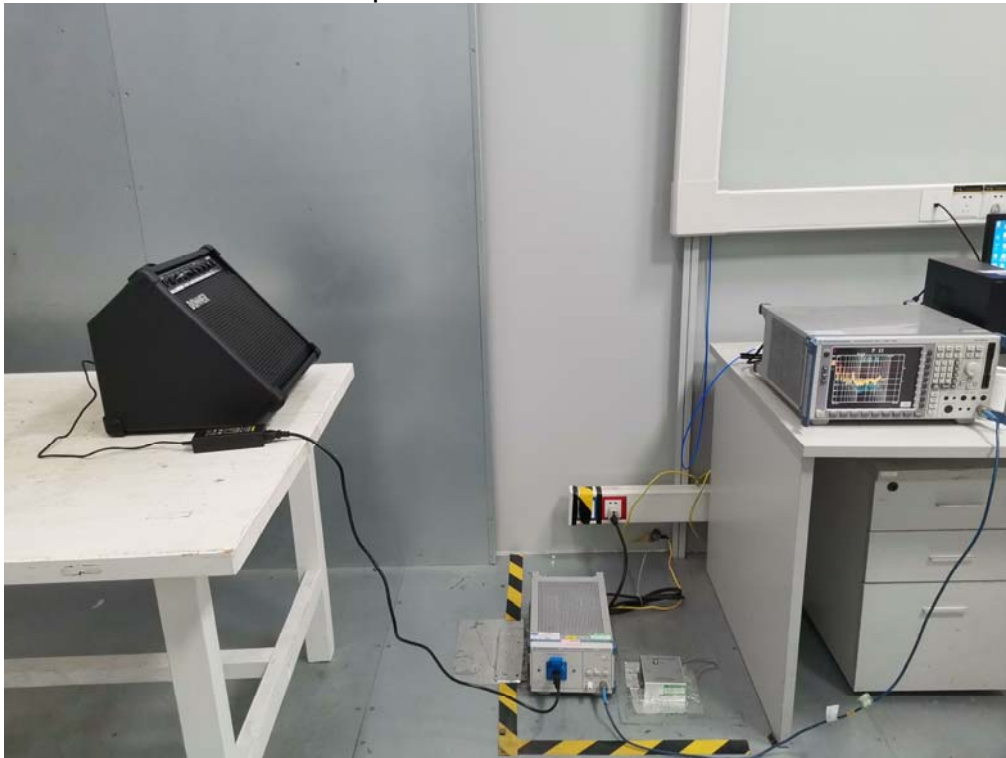
Photos of radiated emission test 30MHz – 1GHz
