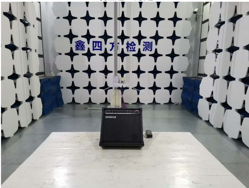
Photos of radiated emission test 30MHz – 1GHz
