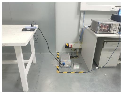
Radiated emission test 30MHz – 1GHz
