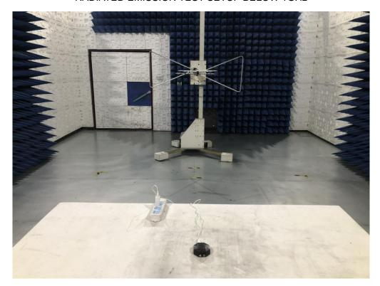
RADIATED EMISSION TEST SETUP ABOVE 1GHz
