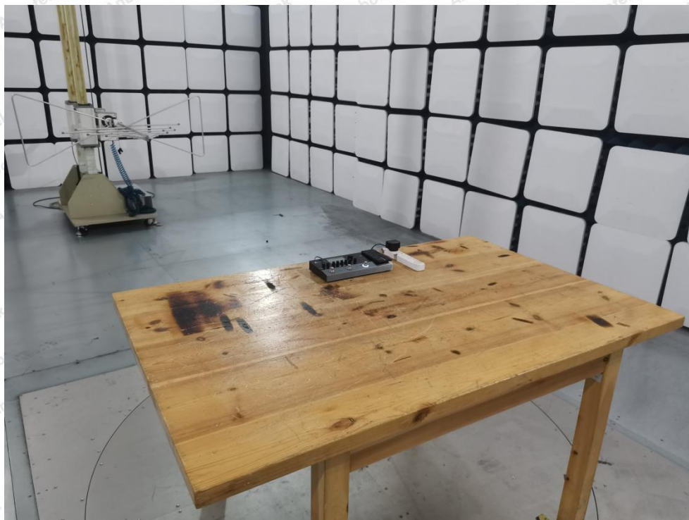
Photo of Radiation Emission Test
