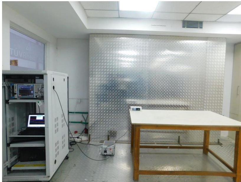
Conducted AC Powerline Test Setup
