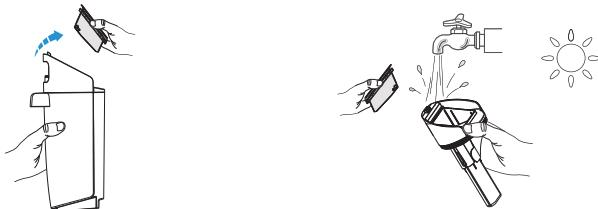
Grasp recessed area on each side of the HEPA and pull upward. Rinse under running water and must be completely dry before recombining with the lid of the DWT.
