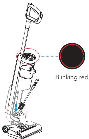
When LED loop blinking red, remove Dirty Water Tank, clean the dirt sensor with a damp cloth or 3-in-1 cleaning tool.
