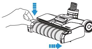
Remove hair and debris from the brush roller chamber and the opening with a tissue or a damp cloth.
