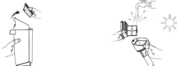
Grasp recessed area on each side of the filter and pull upward. Rinse under running water and must be completely dry before recombining with the lid of the DWT.
