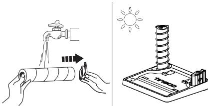
Remove the hair and debris wrapped around the roller and rinse with water (brush roller tab can be removed). Replace the brush roller back onto the storage tray, and allow it to dry completely before reinstalling.
